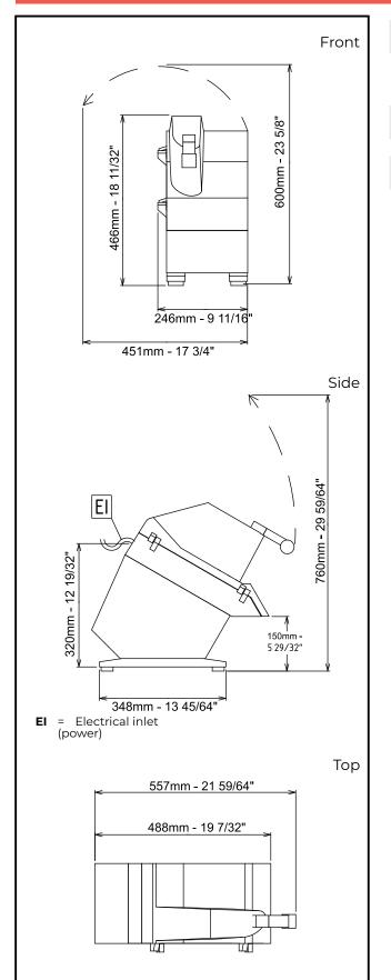
Electric Supply voltage: 220 V/1N ph/60 Hz Electrical power, max: 0.37 kW 0.37 kW **Total Watts:** Capacity: Performance (up to): 550 kg/hour Key Information: External dimensions, Width: 246 mm External dimensions, 557 mm Depth: External dimensions, Height: 466 mm **Shipping weight:** 22 kg
